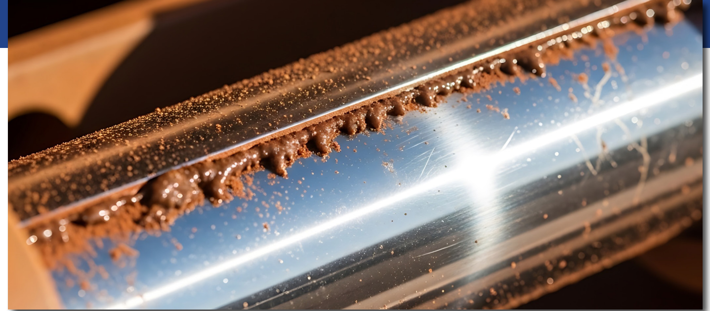
A corroded hydraulic cylinder shows signs of rust and wear.
