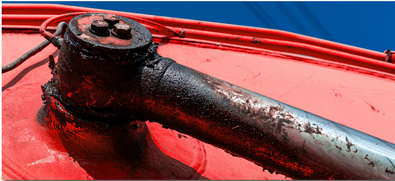
Hydraulic cylinder linkage showing grease leakage.
